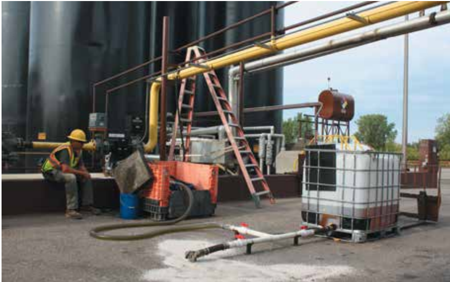
Adding rejuvenator at a commercial asphalt plant during a test-and-control project with RAP.
