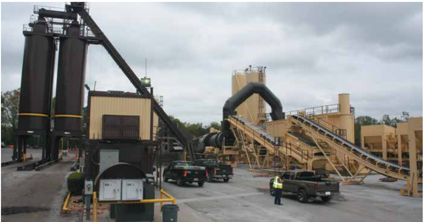
NAPA Member C.W. Matthews assists in reducing RAP stockpiles in the state of Georgia by increasing RAP percentages in its mixes.
