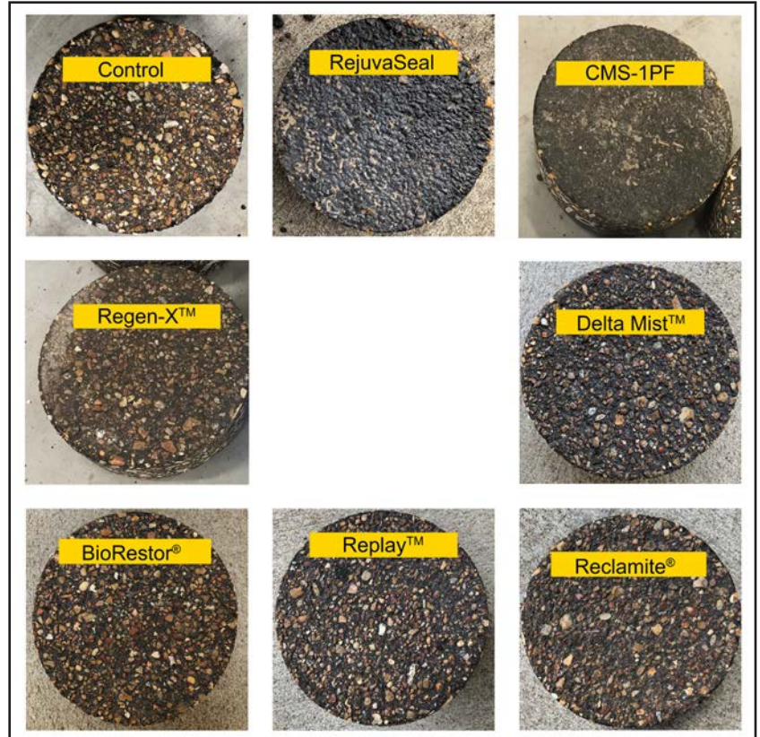
Surface of extracted cores from the NCAT preliminary study four weeks after application of the rejuvenating fog seal treatment.
