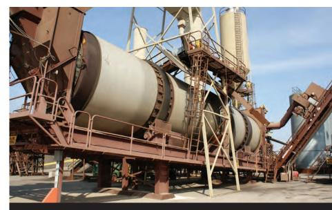
The Delta-S rejuvenator is blended inline at a rate of about 1.5 pounds per finished ton, which Nolan described as "an exceptionally small amount." For the Hennepin County project, Commercial Asphalt Company loaded out the material at temperatures between 290 and 300 degrees F
