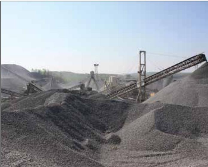
Tilcon employees move blasted and drilled aggregate product to the start of its crushing process and initial crushing piles in the quarry operations in Wharton, New Jersey.
